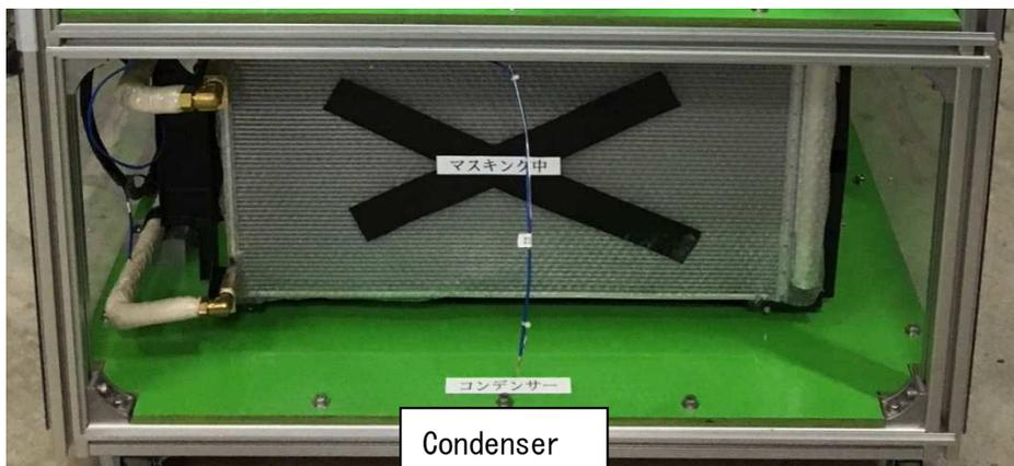
Note2) In order to suppress the function of heat exchange, the surface of the condenser is masked.
